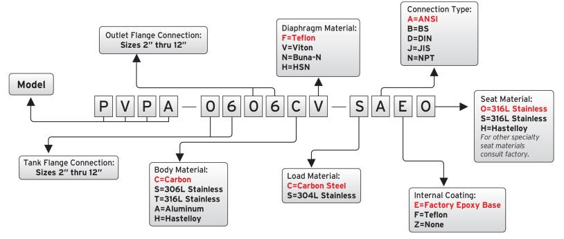
Example: The above order number indicates a Pressure vent with Pipe-away construction. Tank Flange connection is 6", Outlet is 6", Carbon Steel body, Viton diaphragm, Weight loaded with Steel weight material, and Factory Epoxy Base Internal Coating.
